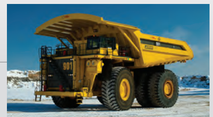
HT-930E-OB-1000 – Komatsu 930E (320 ton payload) SMS curved canopy design. Location: Fort McMurray, AB
