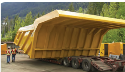
HT-930E-OB-1000 – Komatsu 930E (320 ton payload) SMS curved canopy design. Location: Fort McMurray, AB
