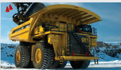
HT-930E-OB-1000 – Komatsu 930E (320 ton payload) SMS curved canopy design. Location: Fort McMurray, AB
