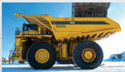
HT-930E-OB-1000 – Komatsu 930E (320 ton payload) SMS curved canopy design. Location: Fort McMurray, AB
