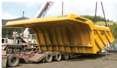
HT-930E-OB-1000 – Komatsu 930E (320 ton payload) SMS curved canopy design. Location: Fort McMurray, AB
